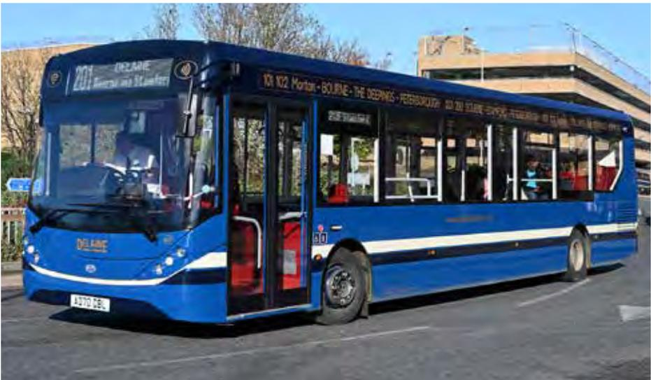
The newest vehicle in the Delaine Buses fleet is 167 (AD70DBL), an 11.8m ADL Enviro 200MMC - the first of its type for the Lincolnshire-based operator. It will be followed in 2021 by a second example. © Steven Knight Media
